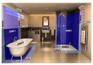
**NOTE:** In the case of bathroom installations, electrical regulations prohibit the installation of Mains Voltage products such as thermostats, contactors, fused spurs, isolators or junction boxes, within Zones 0 or 1.
